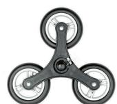
The wheels can be removed without using any tools. To remove the wheel, simply pull it from the rack with the wheel spring pressed down. For better running capacity and longer durability, the bushings can be lubricated with grease at regular intervals (e.g. with clear silicone spray, white Teflon grease).
